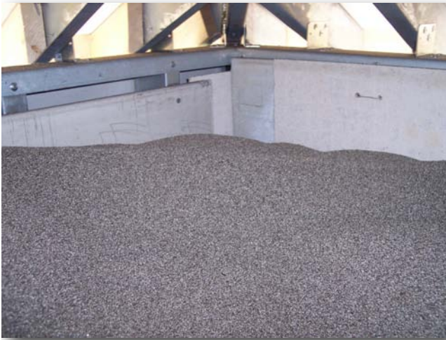
13.4 Loose vermiculite fills a walled enclosure.
