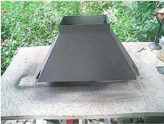
10.1. A fabricated metal vent.
